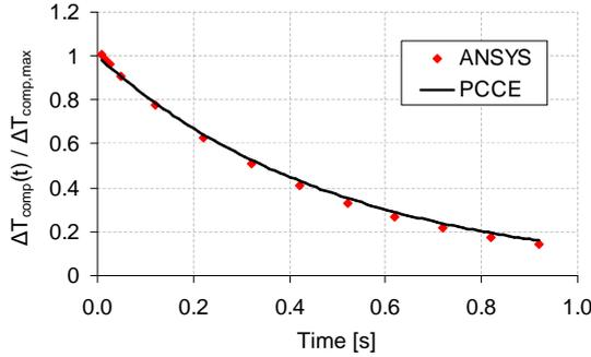
Figure 3: Benchmark of PCCE against ANSYS<sup>®</sup> (transient analysis with a tridimensional finite element model).  $\Delta T_{comp}$  is equal to the difference between  $T_{comp}$  and  $T_{fluid}$ . A good agreement can be observed between the two codes.
