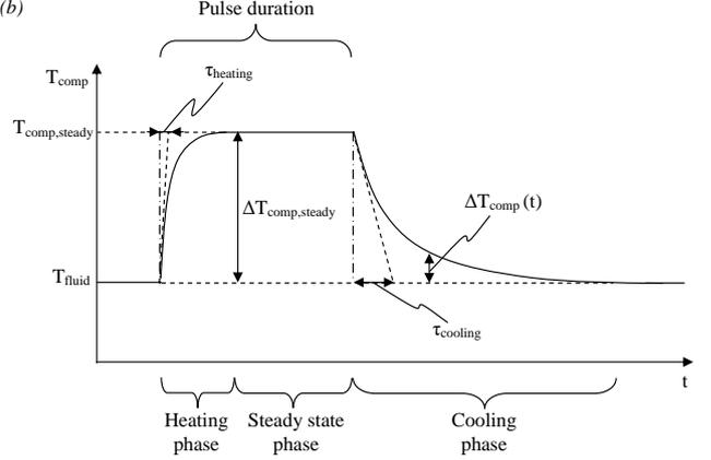
Figure 2: Simplified model of heat exchange inside an actively cooled component: (a) Equivalent electrical scheme; (b) Time behaviour of component average temperature.
