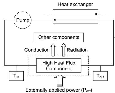
Figure 1: Cooling scheme of a generic high heat flux component.
