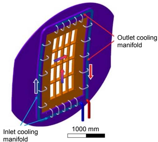
Figure 3. GG assembly view with cooling scheme
