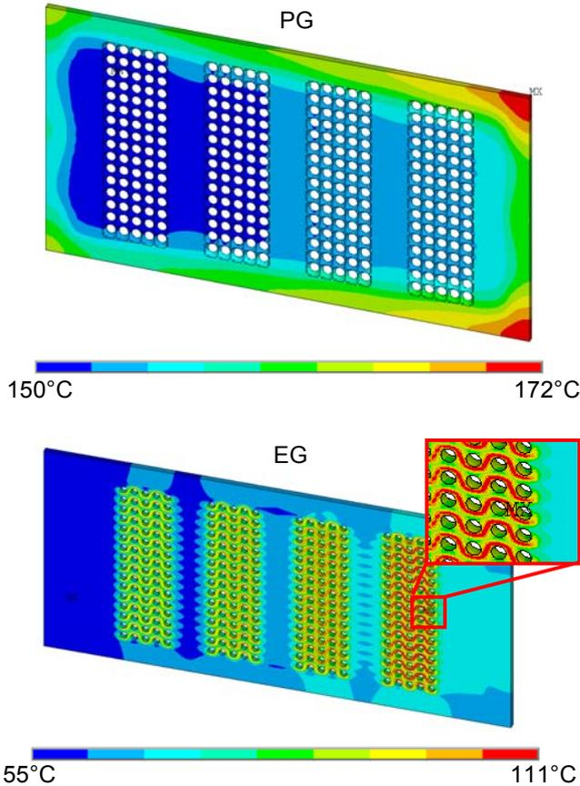
Figure 6. PG and EG temperature contour plots, under nominal power
