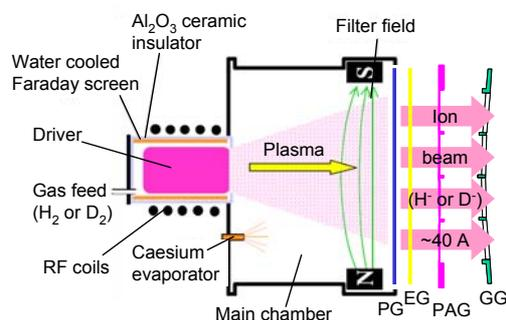
Figure 1. Beam source sketch with RF source and SINGAP accelerator
