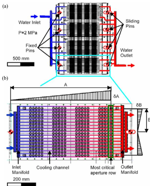
Figure 4. PG, EG and PAG cooling and positioning scheme: (a) Whole grid; (b) Segment
