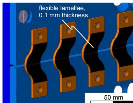
Figure 5. Typical flexible connection between PG segments
