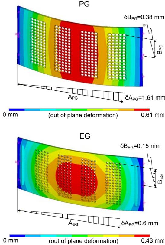
Figure 8. PG and EG deformations, under nominal power (reference temperature of 20°C is assumed)
