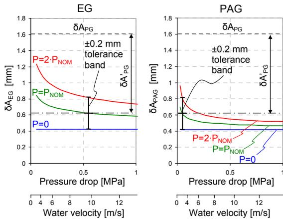
Figure 9. Identification of PG apertures pre-offset and of the minimum EG and PAG cooling parameters for alignment optimization
