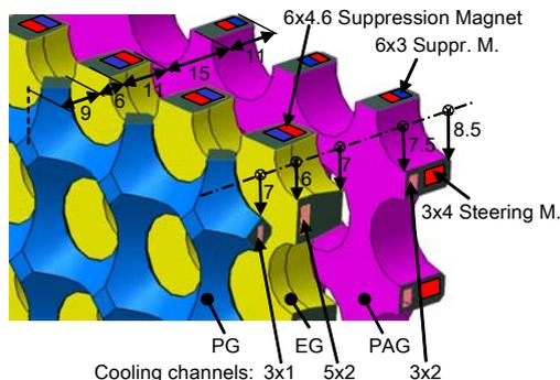
Figure 2. PG, EG and PAG detail (dimension in mm)
