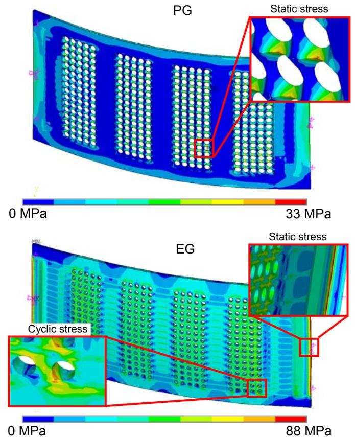
Figure 7. PG and EG equivalent (Von Mises) stress contour plots, under nominal power
