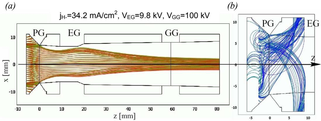
**FIGURE 4.** Beam simulations with BYPO: (a) Trajectories of  $H^-$  with  $\alpha_s = -0.1$  rad (red),  $\alpha_s = 0$  rad (brown),  $\alpha_s = 0.1$  rad (green); (b) Trajectories of coextracted electrons
