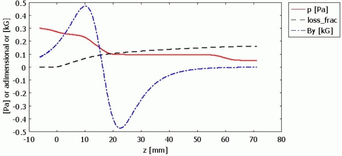
**FIGURE 3.** Profile of the gas pressure, of the stripping losses (loss\_frac) and of the magnetic field vs  $z$  computed with BYPO
