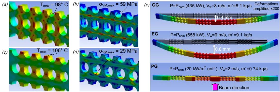
**FIGURE 8.** Main results of the thermo-structural analyses performed with the ANSYS code on the reference scenario: (a) and (b) Temperature and Von Mises equivalent stress on the EG; (c) and (d) Temperature and Von Mises equivalent stress on the GG; (e) Out of plane deformations of the three grids.
