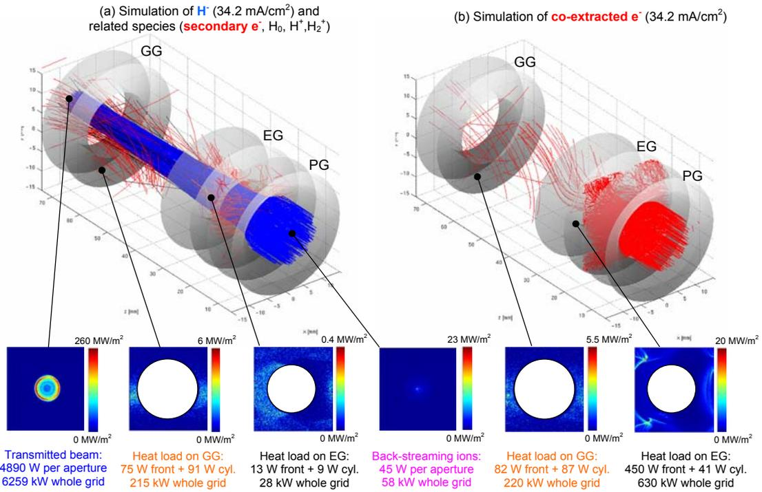
**FIGURE 6.** EAMCC simulation of the beam: the particle trajectories and stripping reaction are simulated with a Monte Carlo approach in a domain with electrical and magnetic fields. For the grids, the heat loads on the front surface (front) and on the cylindrical part (cyl.) are reported for a single aperture, as well as the load on the whole grid. For the transmitted and backstreaming beams, the power corresponding to a single aperture and the total power are reported.
