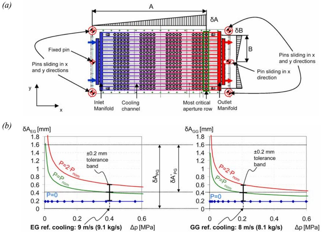
**FIGURE 7.** Alignment optimization for grids: (a) Cooling and fixing scheme; (b) In-plane deformation plots with identification of PG apertures pre-offset and of the minimum EG and GG cooling parameters. The nominal power is the sum of the power given by the secondary, stripping and co-extracted electrons, as calculated by the EAMCC code in the reference operating scenario (full power and 1:1 electrons-to-ions ratio)
