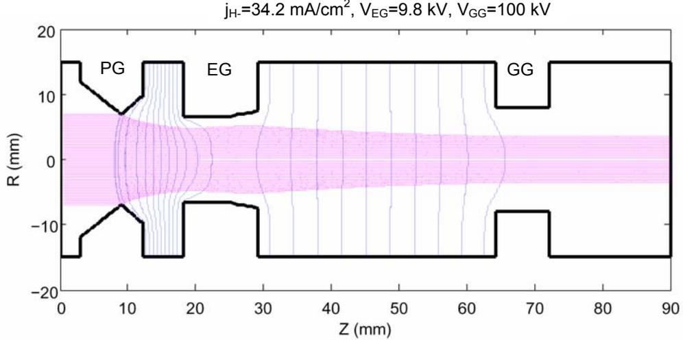
**FIGURE 2.** SLACCAD simulation of the beam optics: equipotential lines (blue) and particle trajectories (magenta) are estimated by integration of the Poisson's equation
