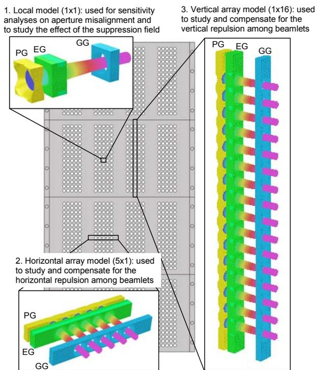
Figure 2. Models of the SPIDER extractor/accelerator system used for the investigations on beam optics and aiming.
