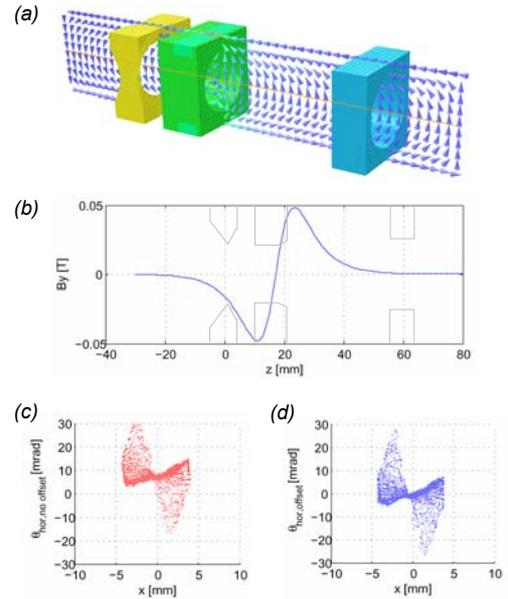
Figure 5. Magnetic field compensation: (a) Magnetic field vector plot in the analysis domain; (b)  $B_y$  field along the beamlet axis (c) Horizontal divergence, without offset. A horizontal deflection of 8 mrad rightward is observed; (d) Horizontal divergence, with offset. The beamlet deflection due to the magnetic field is compensated by a 1mm offset of the GG aperture rightward.
