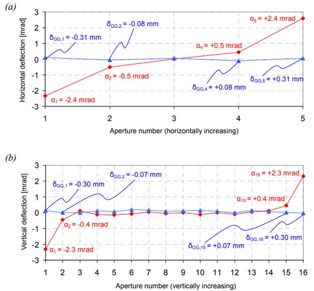
Figure 4. Beamlet repulsion compensation: (a) Horizontal deflection compensation; (b) Vertical deflection compensation. The red dots represent the beamlet deflections due to the interaction between beamlets; deflections angles for each beamlet are reported in red. The blue dots represent the beamlet deflections after introducing proper offsets to the GG apertures, that compensate for the repulsion between beamlets; the optimized values of the aperture offsets are reported in blue.
