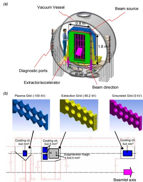
Figure 1. Scheme of the grids for the SPIDER extractor/accelerator system: (a) Design overview; (b) Detailed view of the grids.
