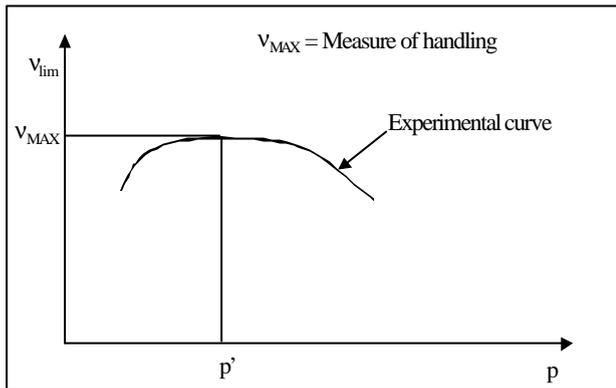
Fig. 15 Definition of a new index to measure the handling of a motorcycle
