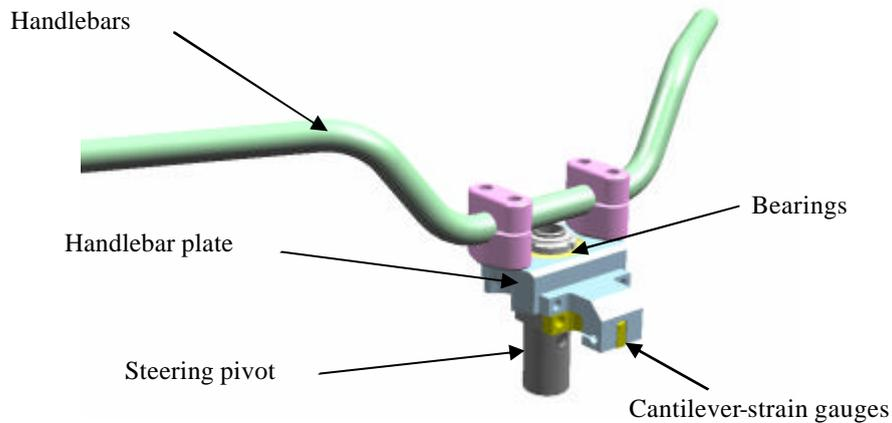
Fig. 6 Steering torque transducer
