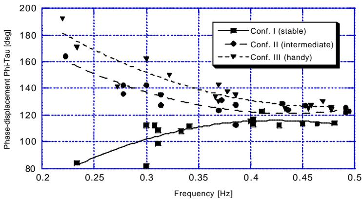
Fig. 10 Phase-displacement  $j-t$  with the three configurations of the quadrilateral in 14m-step slalom
