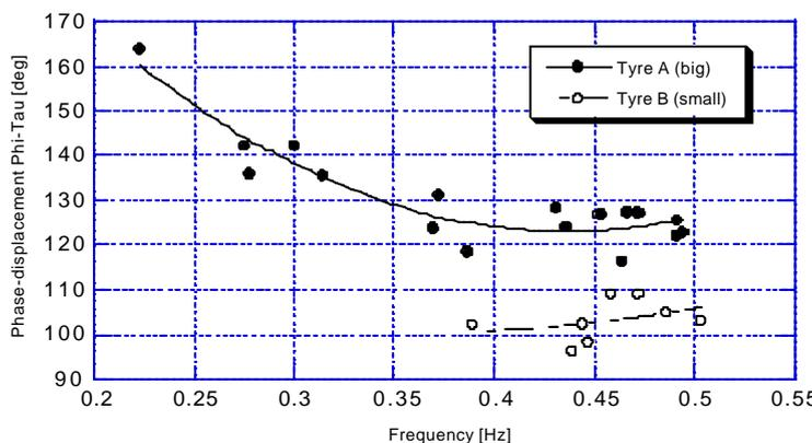
Fig. 12. Phase-displacement  $j-t$  with the two front-tyres in 14m-step slalom
