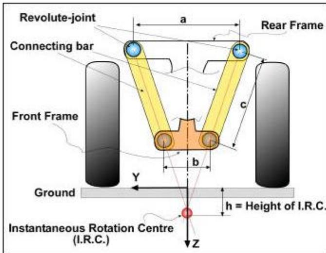
Fig. 3 Four bars linkage elements.
