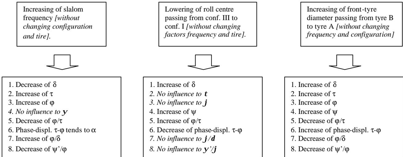
Fig. 13. Synthesis of the influence of the three factors to the significant parameters
