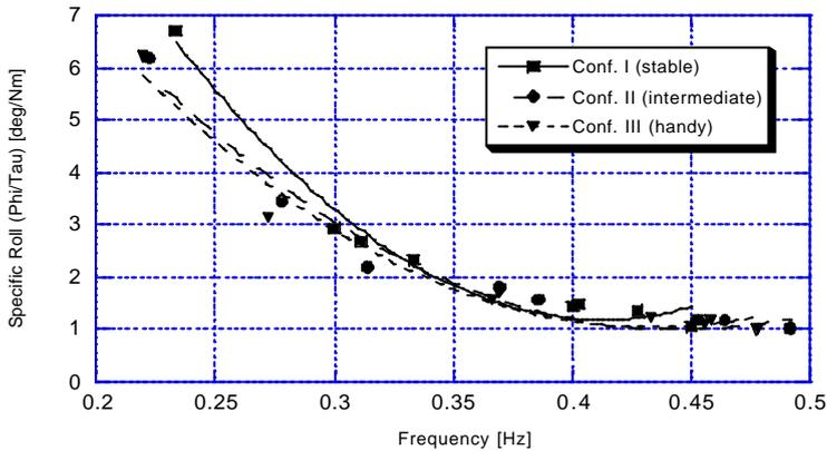
Fig. 9 Specific roll with the three configurations of the quadrilateral in 14m-step slalom
