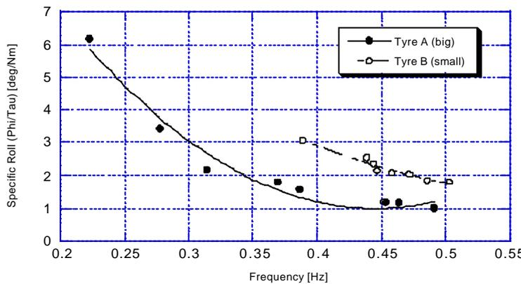
Fig. 11 Specific roll with the two front-tyres in 14m-step slalom
