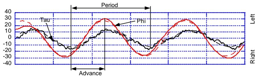
Fig. 8 Phase-displacement between  $\tau$  and  $\phi$ : example of a 7m-step slalom
