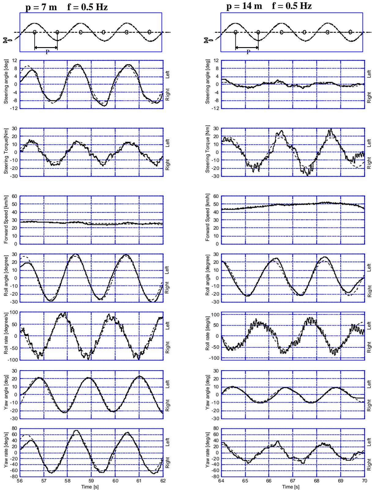
Fig. 7 Acquired data, cones spacing 7 and 14 m, frequency 0.5 Hz
