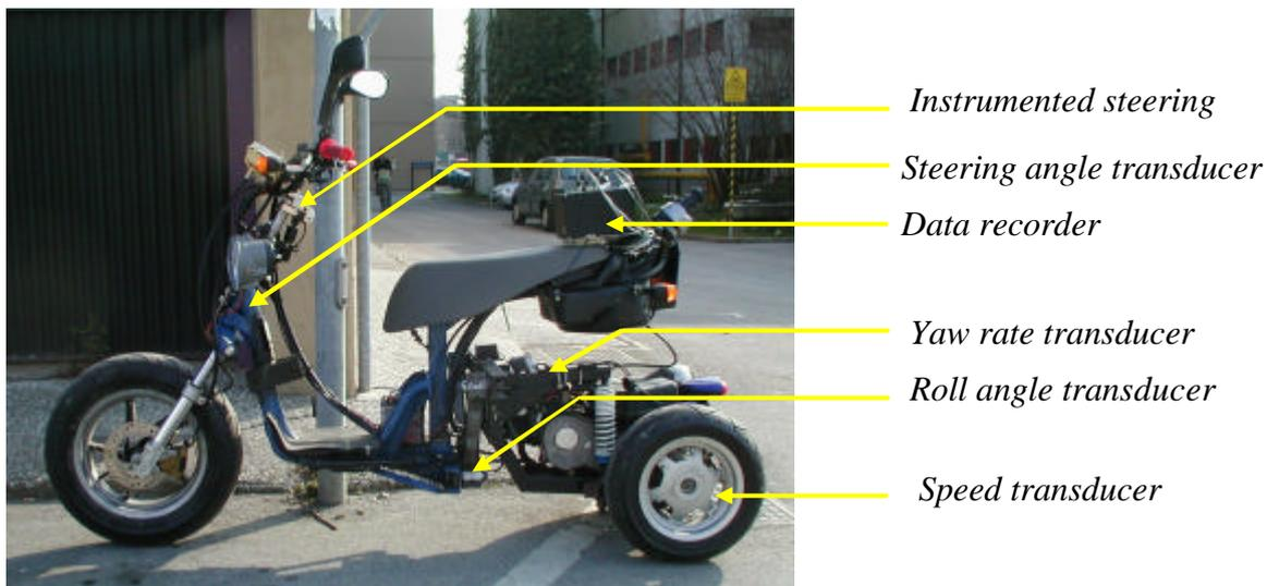
Fig. 5 Data acquisition system
